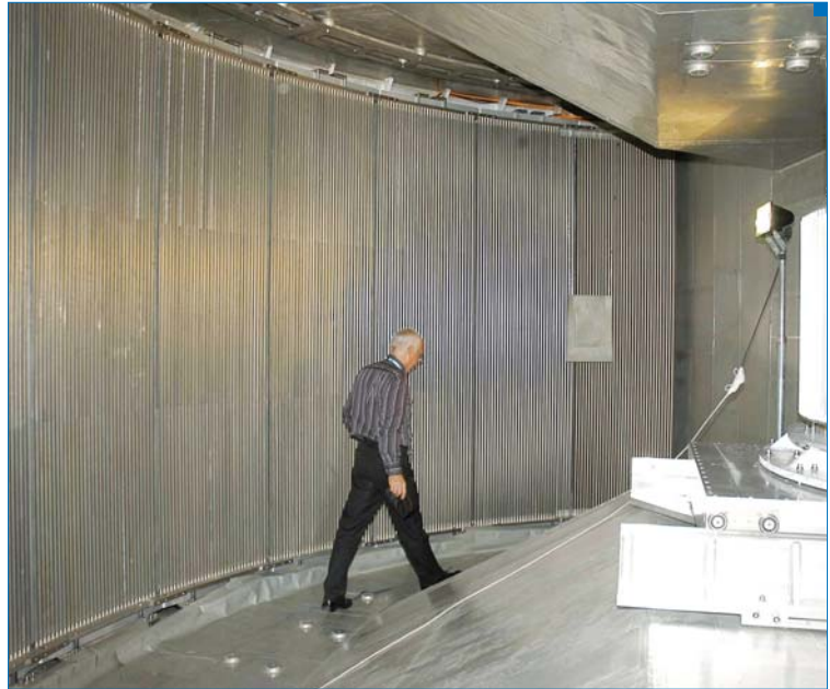
Figure 1: The 3 m-long tubes of the IN5 detector welded on the flange with the orbital weld head.
