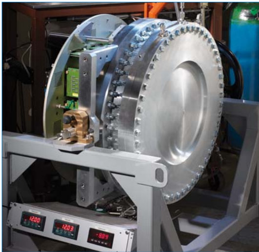
Figure 5: The MILAND detector undergoing tests in the detector laboratory.
