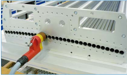
Figure 1: The 3 m-long tubes of the IN5 detector welded on the flange with the orbital weld head.
