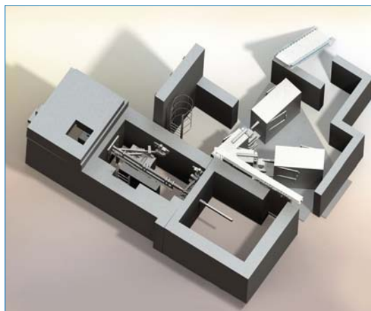
Figure 7: View of the instrument housing for the SuperADAM project showing the high and low resolution configurations.
