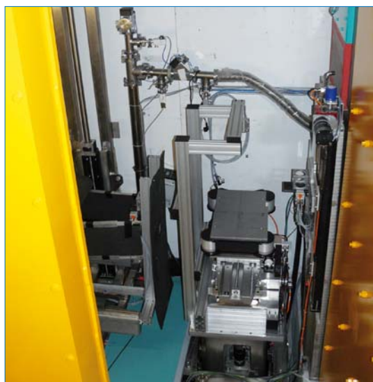
Figure 2: Sample area: The goniometer is visible on top of the vertical translation rig. The yellow lead door is closed during measurements.
