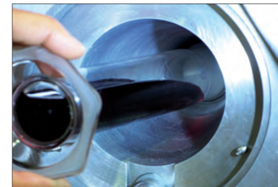
Figure 4: The Moses effect inside the room temperature bore. The diamagnetism of water and alcohol (the tube contains red wine) causes the liquid to be repelled, bringing about the 'parting of the red wine'.
