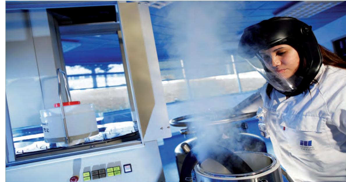
Addition of nitrogen on a gamma spectrometer in the environmental laboratory.
