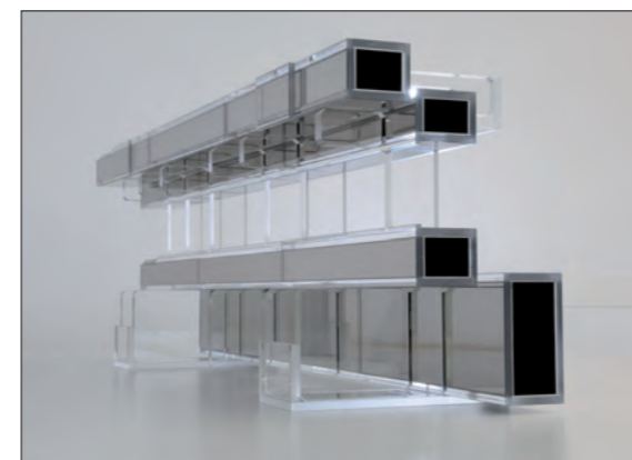
Figure 3: Elements of the H14 neutron guide. The lower part goes to IN12 and D33 and the upper part to LADI and IN11 .
