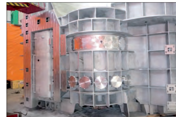
Figure 4: Main aluminium vacuum chamber for IN16B .
