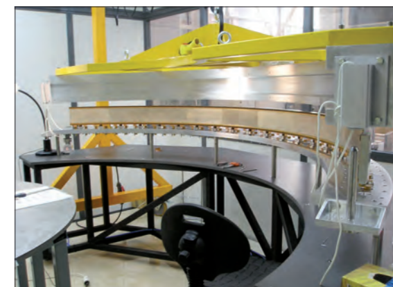
Figure 5: New detector for D1B covering a scattering angle of 130 degrees.
