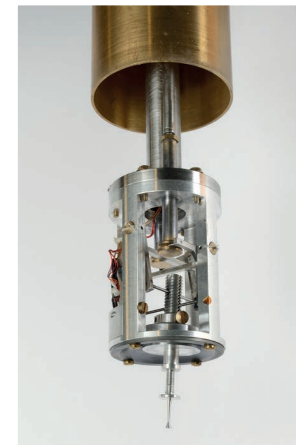
Figure 3 Photo of the Goniosstick with the sample holder inclined by both levers. (© Ecliptique – Laurent Thion).
