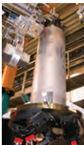
An as-cast aluminium billet for stress determination on SALSA
