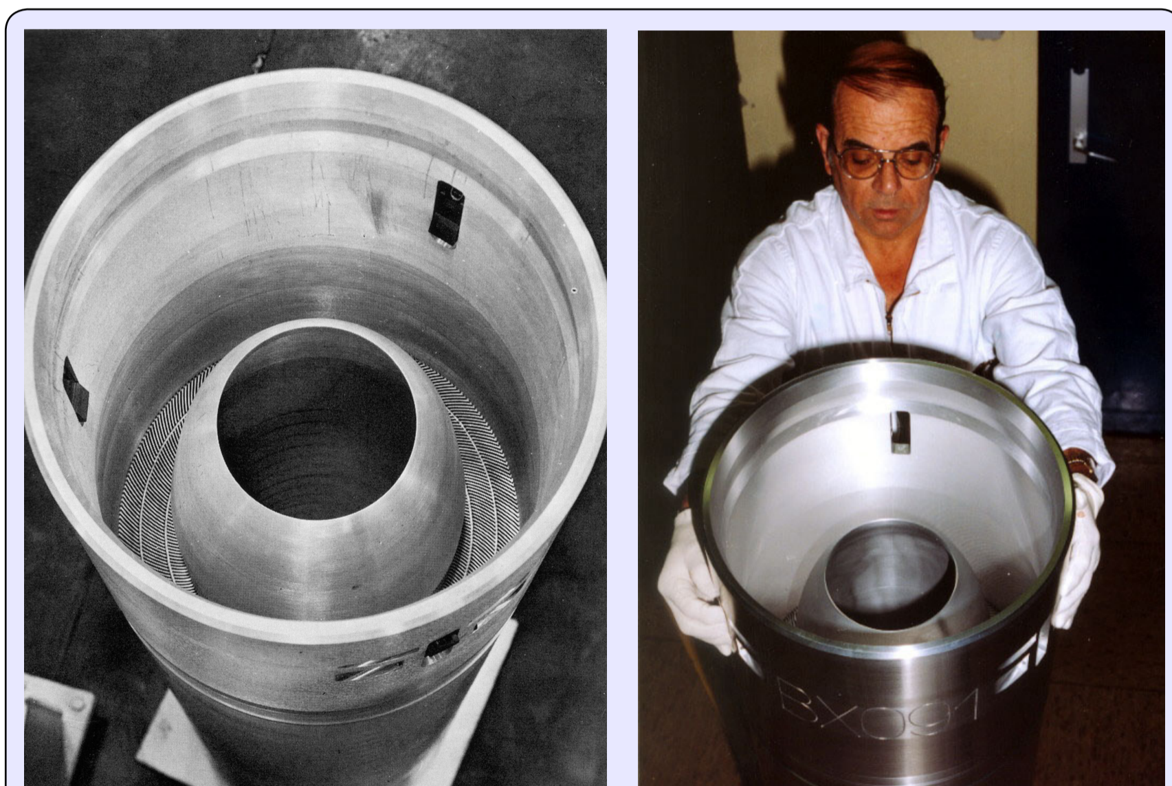
Fig. 5.6: The fuel element. The control rod occupies the central space. The uranium is in the fins between which circulates the heavy water coolant.
