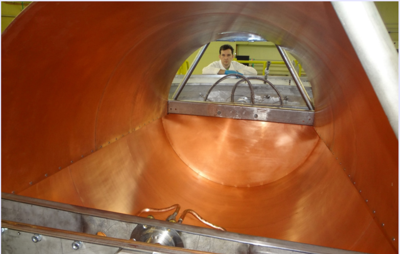
Fig. 11.10: GraviTrap, a gravitational trap for ultra cold neutrons (UCNs) for the measurement of the neutron lifetime. The bathtub like trap coated with a special grease impervious to UCNs is here in the bottom of the enveloping copper cylinder. The UCNs accumulate in the trap as the atoms of a heavy gas would due to gravity. The trap can be horizontally rotated to empty it by pouring out the UCNs.
