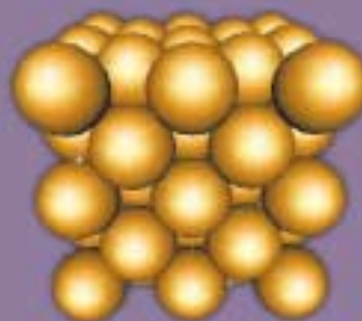
The structure of gold, revealing its 'stack of oranges' arrangement
