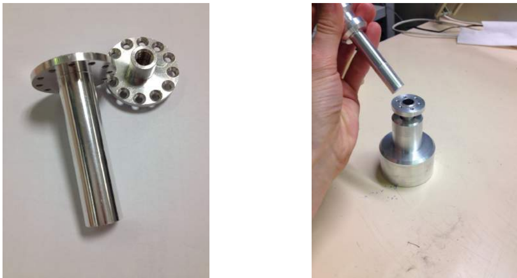
FIGURE 2.10: Left: Photo of a cylindrical Aluminium sample holder used during the experiment on IN1-Lagrange. Right: Photo of a cylindrical Aluminium sample holder, placed into an apposite metal support for gently pressing the sample inside.
