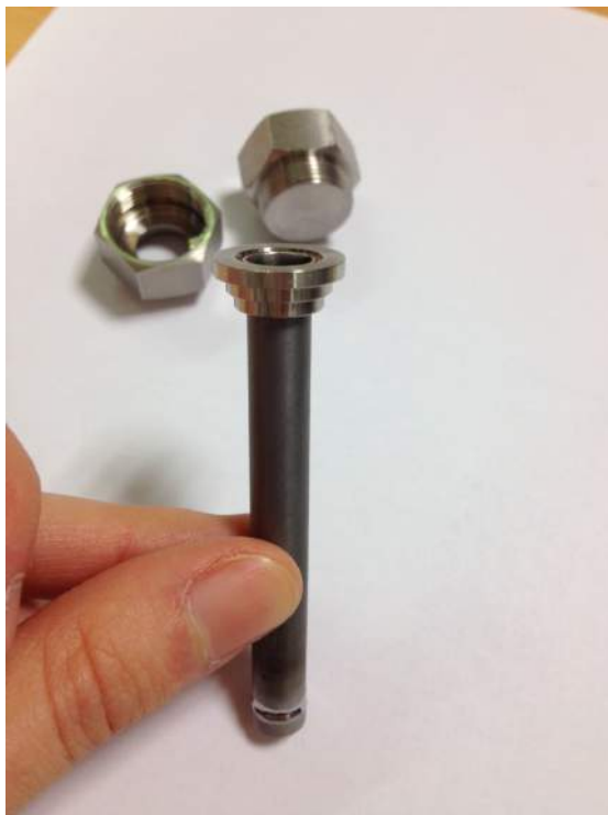
FIGURE 2.3: Image of a typical 7mm Vanadium cylindrical sample holder used during the experiment on D4C.
