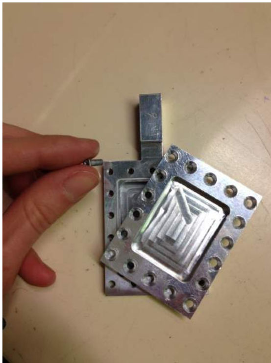
FIGURE 2.4: Image of a flat Aluminium sample holder used during the experiment on IN4C.
