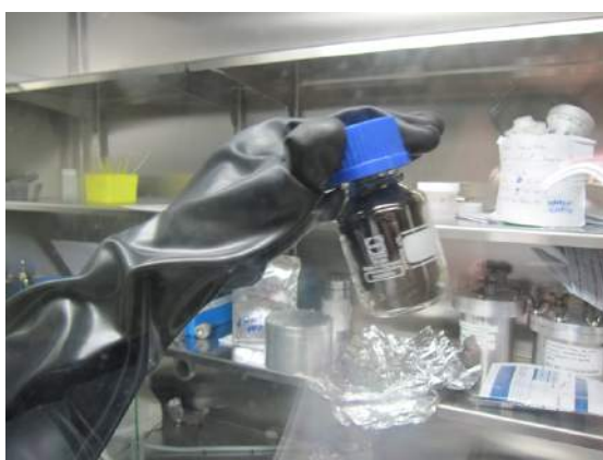
FIGURE 2.5: Image of vial containing TEGO powder for an the experiment on IN4C. Sample handling and manipulations were done inside a glovebox in order to prevent any possible oxygen moisture contamination of the samples.
