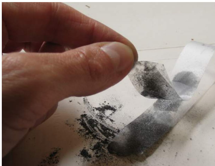
FIGURE 1.7: Sticky tape can be used to peel off powdered graphite, leaving a single layer of graphene. Taken from lostinscience.wordpress.com .
