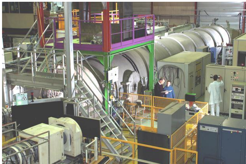
Figure 2.18: Picture of the small-angle diffractometer D22 instrument with its 20 metre long detector tube. Photograph from http://www.ill.eu .
