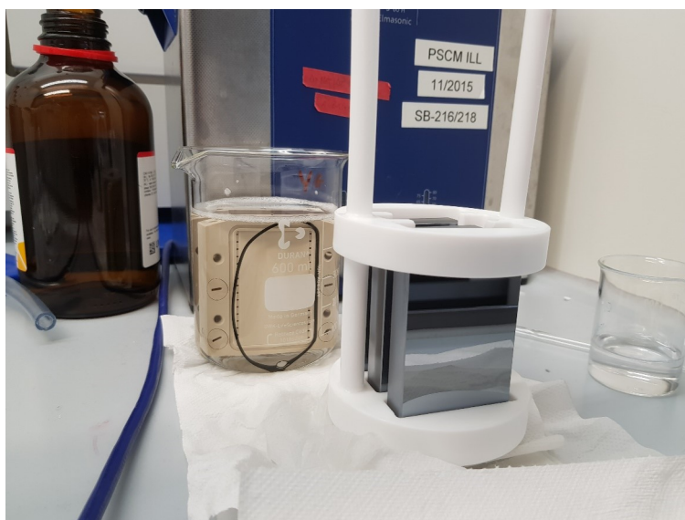
FIGURE A.2: Picture representing the PEEK cells and the silicon crystals used in NR experiments
