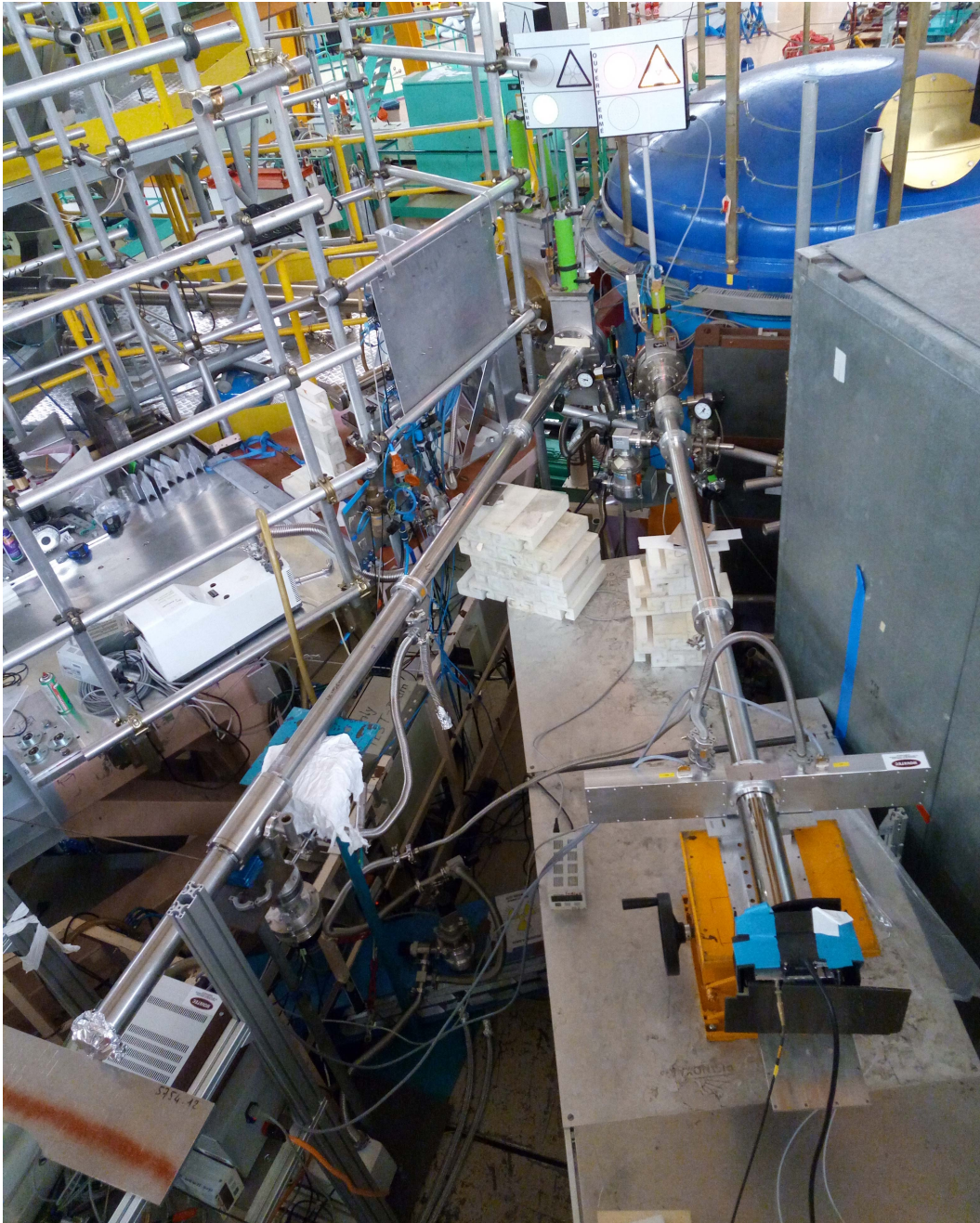
Figure 4.21: The UCN Turbine (blue) is at the top of this image. On the right, the PF2-TEST beamline is shown with the TOF setup used to measure the transmissivity of electropolished, NiMo-coated stainless steel tubes. To the left is the PF2-EDM beamline with its \sim 3 m of electropolished, NiMo-coated stainless steel tubes. The PF2-UCN beamline is located behind the scaffold on the left.
