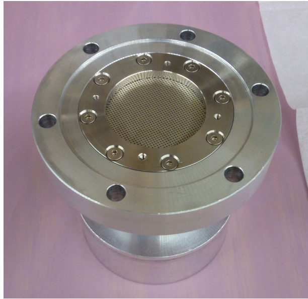
Figure 4.19: Titanium collimator built into the cryostat flange. The aluminum foil that serves as vacuum separator is sandwiched between a protuberance in the flange and the collimator.
