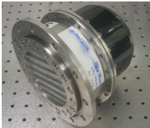
Figure 4.11: View of the Dunya ^3\text{He} proportional detector. Photo by Damien Roulier [148].
