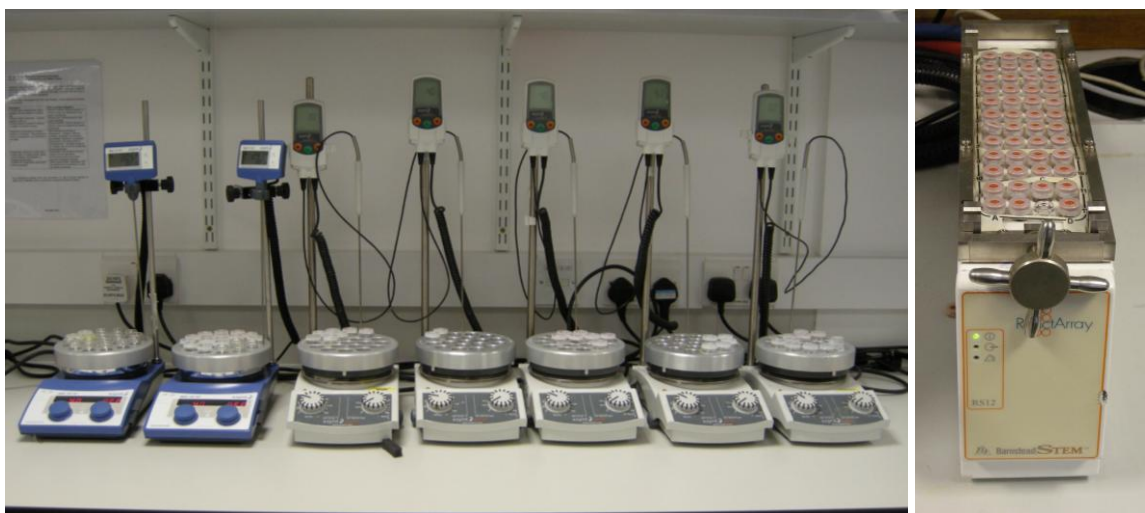
Figure 3.1 Photographs of the temperature controlled hotplates (left) and the ReactArray Microvate (right) used in sample preparation.
