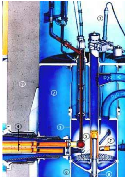
Figure 3.5 Diagram of the ILL reactor core showing: 1. Safety rod; 2. Neutron guide pool; 3. Reflector tank; 4. Double neutron guide; 5. Vertical cold source; 6. Reactor core; 7. Horizontal cold source; 8. Control rod. 148
