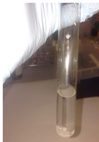
Figure 1: View of the crystals grown in the mono-tube obtained by slow diffusion method.
