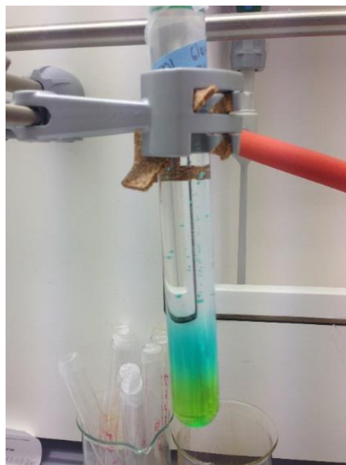
Figure 2: Liquid-liquid diffusion between two methanolic solution. The methanolic solution of a copper salt was layered on top of the methanolic solution of methylamine and formic acid.
