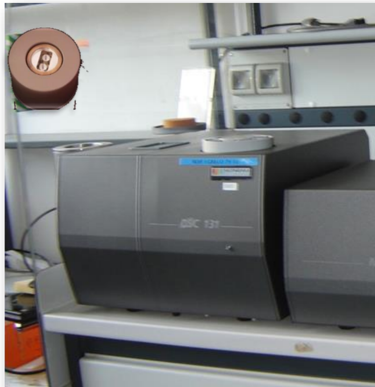
Figure 4: Differential Scanning Calorimeter DSC131 (ILL) and on the left above the typical crucible where lodging the sample.
