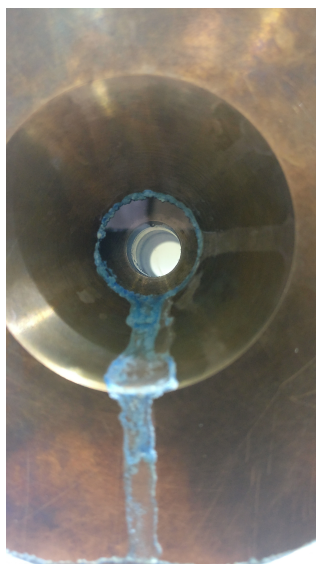
Figure 14: The high pressure cell used for SANS, zoomed at the saffire windows where the beam is transmitted. The picture shows the leakage of material from the windows.
