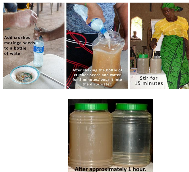
Figure 1.7: Traditional water purification procedure using Moringa seeds – as taught to families in developing countries by the charity association “strong harvest international” (taken from https://www.strongharvest.org/moringa-basics/ ).
