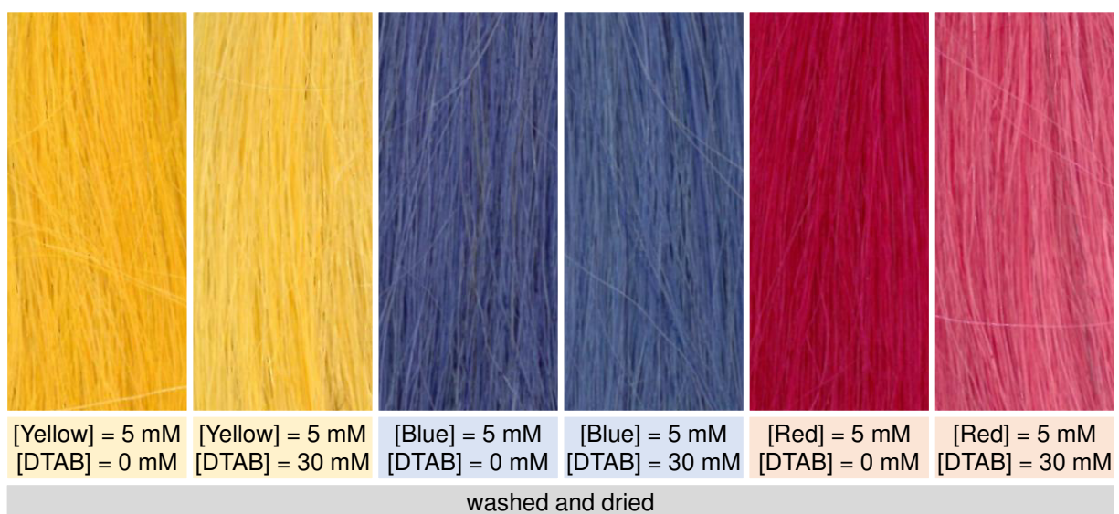
Figure 3: Images of washed goat hair tresses dyed in solutions containing the specified direct dye at a concentration of [Dye] = 5 mM without or with the cationic surfactant DTAB. For each dye, the left image shows the hair tress dyed in absence of DTAB and the right image the hair tress dyed in presence of DTAB. The composition of the dyeing solution is indicated below each image. Dyeing was performed with an excess of dyeing solution and at a temperature of 25 °C for 30 min under constant mixing. A NaHCO 3 /Na 2 CO 3 buffer with pH = 10.5 and an ionic strength I \approx 0.25 M was used as solvent. After dyeing, all hair tresses were washed under running, lukewarm water and subsequently dried using a fan.
