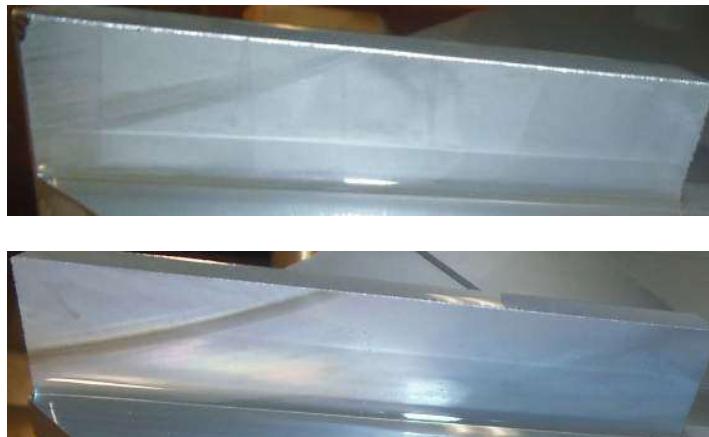
Figure 3.5.: Surface of the cutted (top) and grinded (bottom) interferometer lamella.
