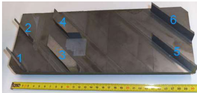
Figure 3.7.: Interferometer after grinding, with blade numbers.
