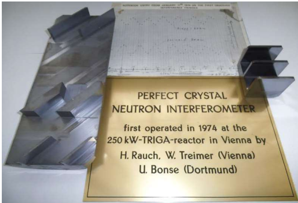
Figure 1.3.: New IFM (left) together with the first Si perfect crystal IFM (right).
