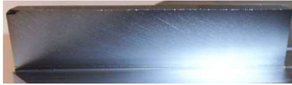
Figure 3.8.: Surface of the etched interferometer lamella from fig. 3.5.
