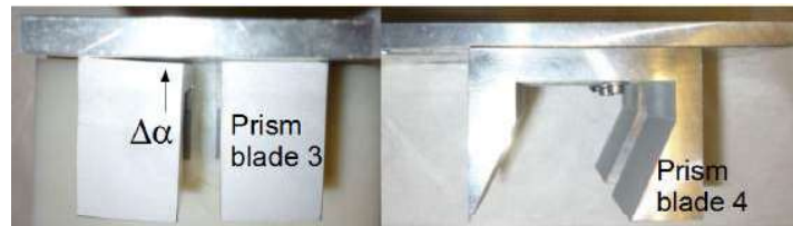
Figure 2.59.: Both prism pairs are mounted over the blades 3 and 4. The blade 4 rotation has a constant offset \Delta\alpha .
