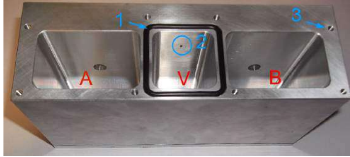
Figure 4.6.: Al chamber system without outer walls. (A)(B) Air chambers ( 65 \times 94 \times 40 \text{ mm}^3 ), (V) vacuum chamber ( 40 \times 94 \times 40 \text{ mm}^3 , wall thickness to (A)/(B) is 8 mm). (1) Vacuum sealing ring, (2) connection to the vacuum system and He-inlet ( \text{\O}5 \text{ mm} hole), (3) screw hole for mounting Al walls.
