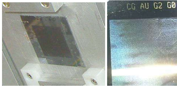
Figure 2.52.: Photography of the used phase diffraction grating with g=16 \mu\text{m} spacing (left) and the absorption diffraction grating with g=17 \mu\text{m} spacing (right).
