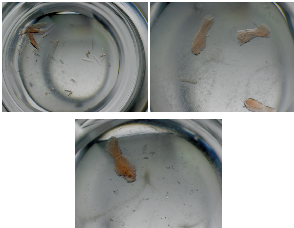
Figure 6.15: Crystals of perdeuterated wild-type ECAO obtained in 1.30 (top left), 1.35 (top right) and 1.4 (bottom) M sodium citrate at pH 7.3 as indicated in table 6.2
