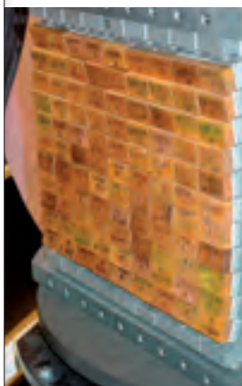
A COPPER CRYSTAL MONOCHROMATOR
