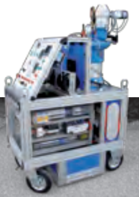
A FULLY AUTOMATED AND MUCH SAFER POWER-RACK FOR THE 20 OR SO FURNACES
