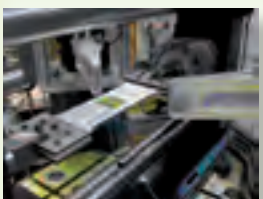
A WELDED PLATE SPECIMEN MOUNTED IN THE SALSA STRESS-RIG (ABOVE); EVOLUTION OF THE RESIDUAL STRESS WITH FATIGUE CRACK-GROWTH (BELOW)
