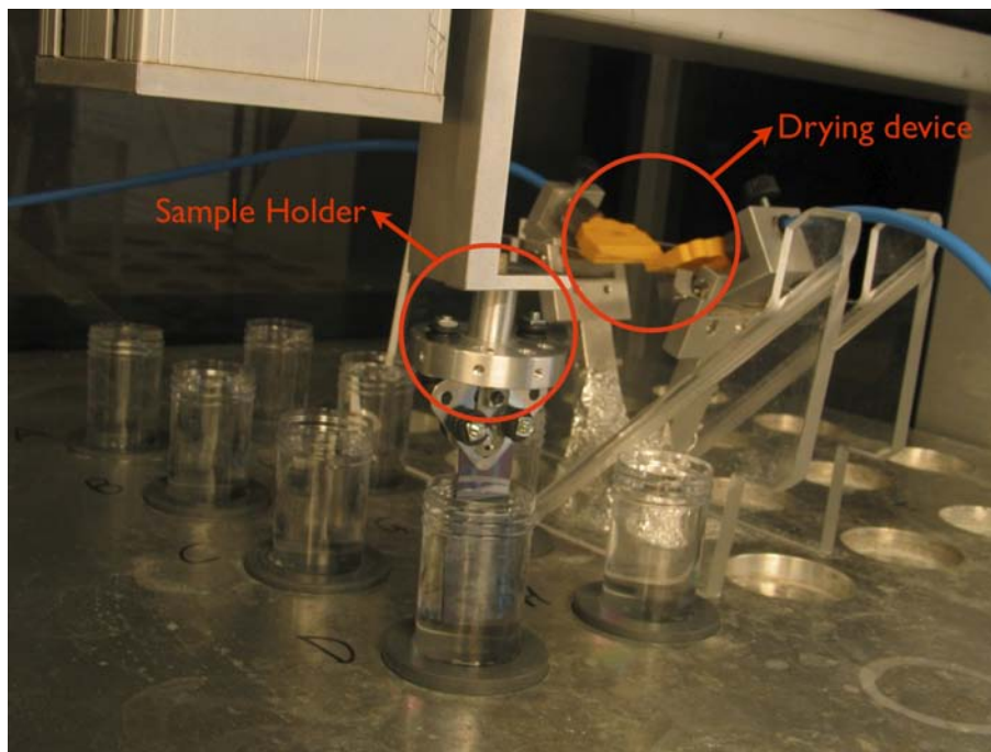
Figure 2.2: Picture of the dipping robot used for the automated dipping.
