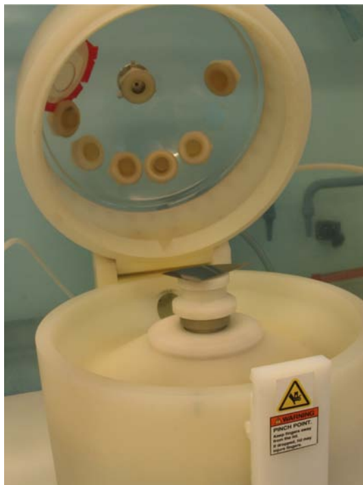
Figure 2.6: Picture of the spin-coater used for the films build-up by using the spin-assisted LbL assembly.
