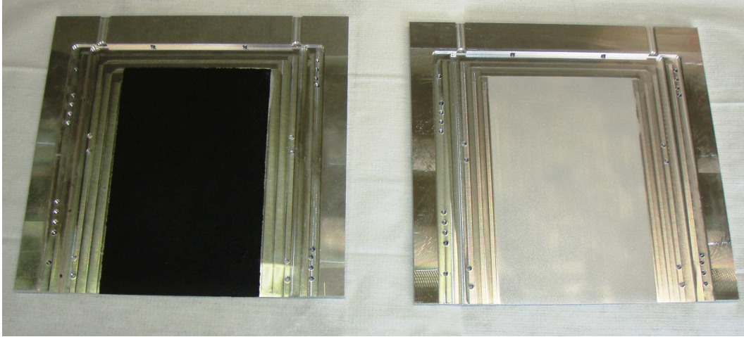
Figure 6.28: A cassette V2 coated and un-coated with ^{10}\text{B} painting.
