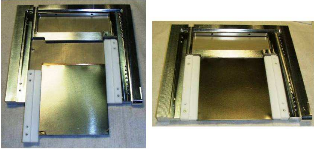
Figure 6.13: The Aluminium holder and a blade (substrate coated with ^{10}\text{B}_4\text{C} both sides) inserted.
