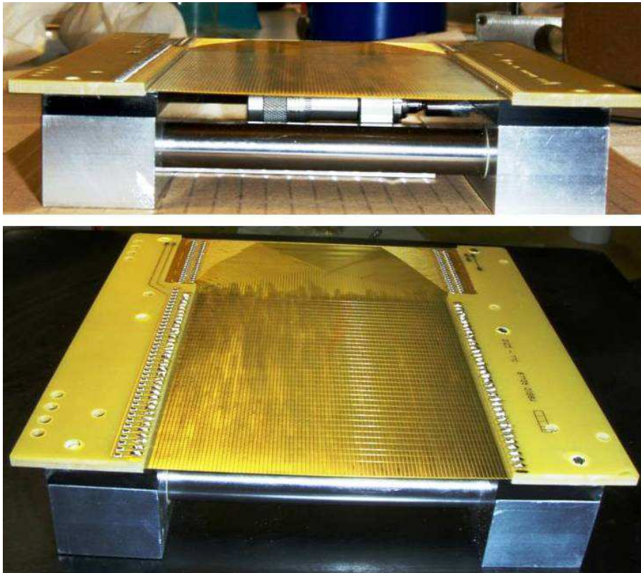
Figure 6.11: A polyimide PCBs where anode wires are mounted orthogonal to the cathode strips.
