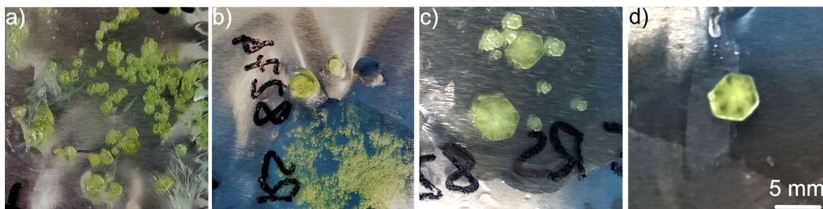
Figure 2.4: Stages of serial seeding recrystallisation for aqueous solutions of [\text{Na}(\text{OH}_2)_3]\text{Mn}(\text{NCS})_3 . Crystals are shown after a) 2 days, b) 5 days and c) 9 days. d) A crystal with a 5 mm scale bar for reference.
