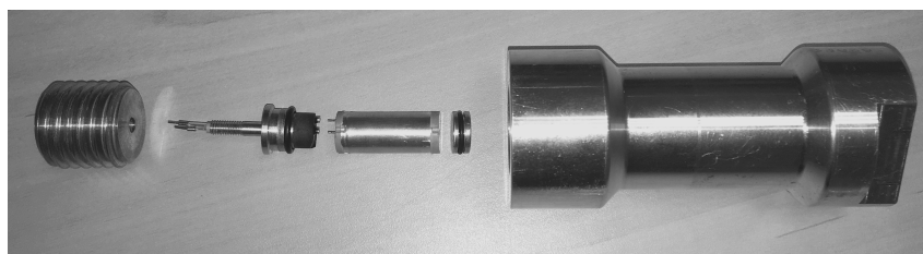
Figure 6.7: The different components of the combined high-pressure dielectric and neutron cell before assembling. The cell is attached to the sample stick from the right, where pressure is applied through the capillary running through the sample stick. The wires from the dielectric setup are attached to the plug at the bottom of the cryostat, this would be on the left here.
