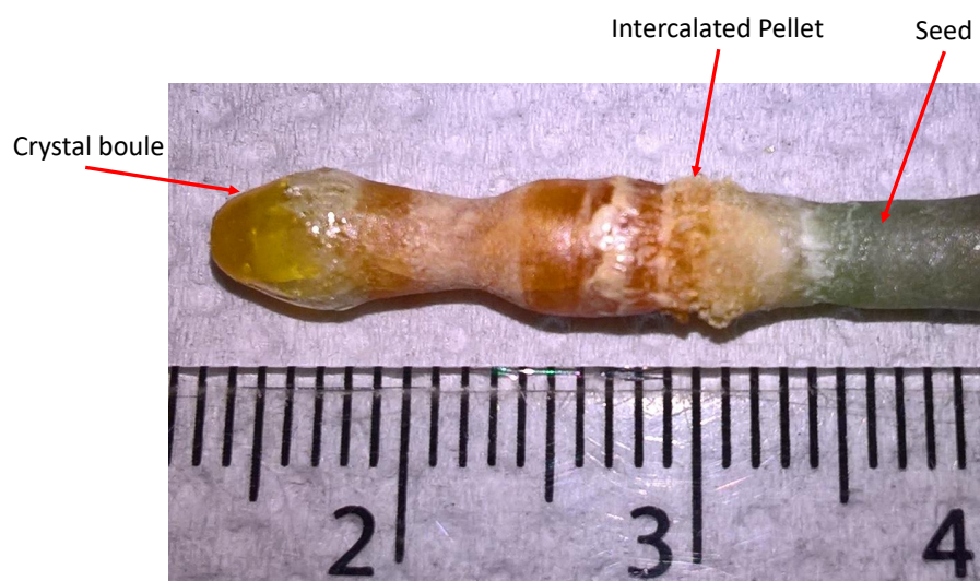
Figure 6.8: Picture of the crystal boule obtained from the single crystal growth of the isotopically enriched \text{SrGd}_2\text{O}_4 material. A small translucent boule containing several single crystal fragments was obtained (left). A principally polycrystalline rod of \text{SrGd}_2\text{O}_4 material containing natural Gd was employed as seed and support for the growth (right). A small pellet of isotopically enriched material was previously melted on top of the seed to act as a spacer preventing for the isotopic contamination of the enriched material.
