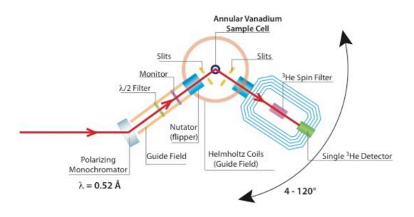
The main limitation of this setup is however the extremely poor Q-resolution resulting from the very small scattering angle of the Heusler (1 1 1) Bragg reflection ( $\theta_{\text{Bragg}} = 4.26^{\circ}$  at  $\lambda = 0.5$  Å) and the fact that the monochromator is used in transmission geometry.
