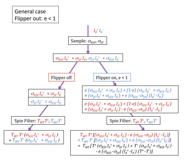
For a nuclear Bragg peak ( $\sigma_{NSF} = \sigma$  and  $\sigma_{SF} = 0$ ) the measured intensities reduce to:
