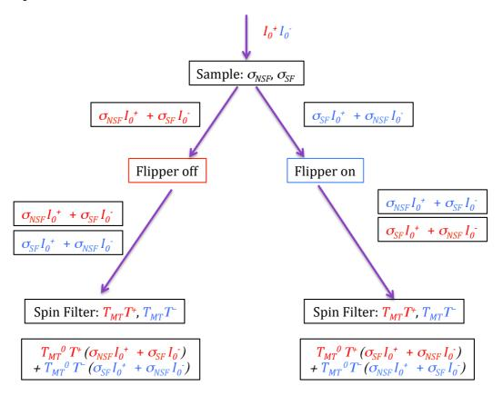
We use  $I_0^{\pm} = T_{MT}^0 I_{in}^{\pm}$ , where  $T_{MT}^0$  is the magic box empty filter transmission.  $T_{MT}^0 = 1$  if there is no magic box (polarization from Heusler monochromator).
