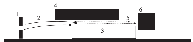
Fig. 1. A principal scheme of the gravitational UCN spectrometer. From the left to the right the following: the vertical bold lines indicate the upper and lower plates of the input collimator (1); the solid arrows correspond to classical neutron trajectories (2) between the input collimator and the entrance slit between a mirror (3, the empty rectangle below) and a scatterer (4, the black rectangle above). The dotted horizontal arrows illustrate the quantum motion of neutrons above a mirror (5), and the black box presents a neutron detector (6). The size of the slit between a mirror and a scatterer is equal to 250 μm, which corresponds to the spread of vertical velocity components of \pm 0.07 m/s.
