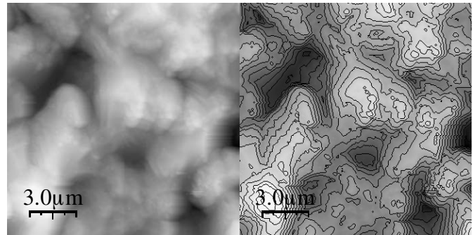
Fig. 2. A typical surface profile of a scatterer with a copper coating, measured using an atomic-force microscope. The maximum height difference between two points here is equal to 2 \mu\text{m} , the distance between neighbouring “hills” is 7 \mu\text{m} .
