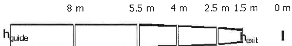
Figure 12: design of a focussing trumpet with quasi-elliptical shape
