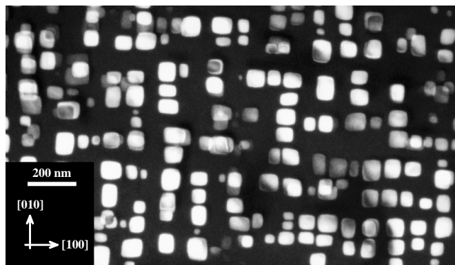
Figure 1 Dark-field transmission electron micrograph of a Ni-12 at.% Al-2 at.% Mo alloy after aging at 1070 K for 10 h.
