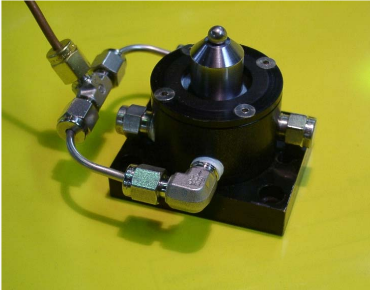
The gas stream levitator nozzle of a levitation system used at the Glass Liquids and Amorphous Diffractometer at the Intense Pulsed Neutron Source at Argonne National Laboratory
