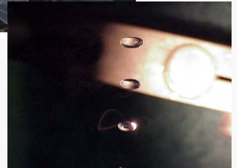
Acoustic levitator with floating water droplet [Y. Cerenius, Å. Oskarsson, S. Santesson, L. Nilsson, L. Kloo, J. Appl. Cryst. 36 (2003) 163]
