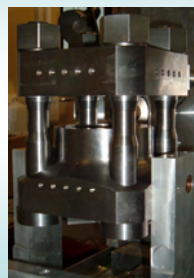
Paris Edinburgh cell. Fibre optic system used for in-situ ruby pressure measurements in safety bunker.
