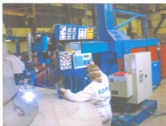
Soudure plasma (CN) – (NC) Plasma arc welding
