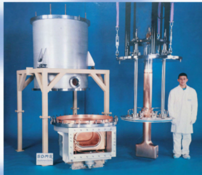
Copper RF-cavity Quarter Wave Resonator 240 kV, 27- 54 MHz
