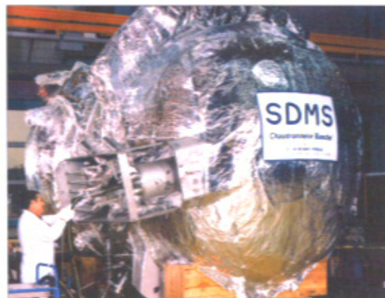
22\text{m}^3 liquid oxygen storage tank during baking
