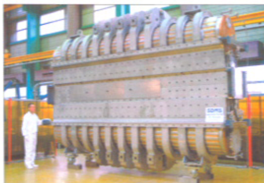
Resonator for 590 MeV Ring Cyclotron. Copper (PSI)
