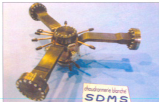
Resonator, stainless steel copper coating (BESSY)
