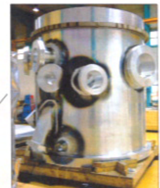
Tank shell after ports welding by electron beam
