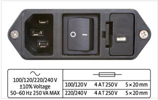
FIGURE 3-2 Line input assembly
