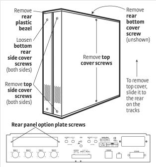
FIGURE 7-3 Cover and option plate screws (full rack)
