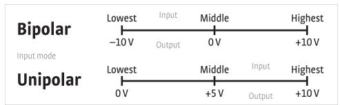
FIGURE 5-2 Unipolar and bipolar mode
