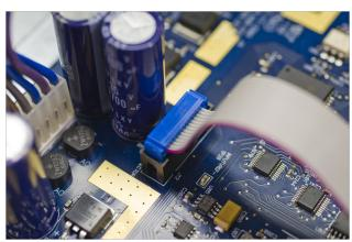
FIGURE 7-4 Proper orientation of the ribbon cable connector plug
