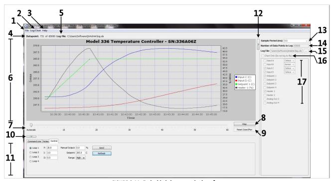
FIGURE 6-11 Embedded chart recorder interface
