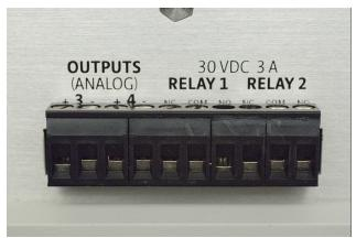
FIGURE 3-10 Output terminal block
