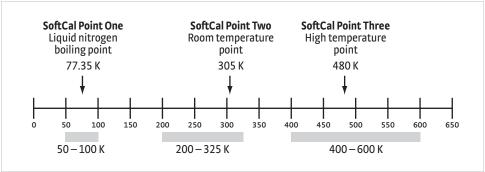
FIGURE 5-9 Acceptable temperature range for platinum SoftCal™ sensors
