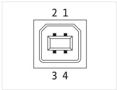
FIGURE 8-6 **USB pin and connector details**
