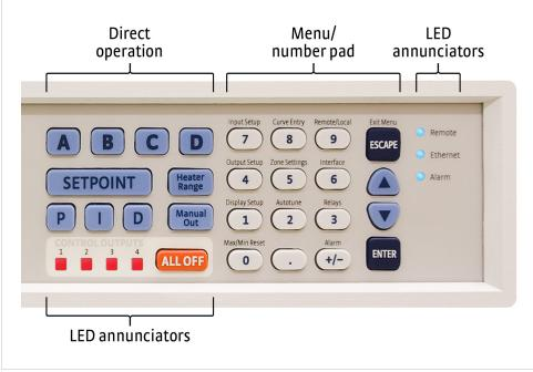
FIGURE 4-1 Model 336 front panel
