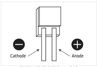
FIGURE 3-4 DT-670-SD Diode sensor leads
