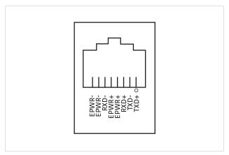
FIGURE 8-7 Ethernet pin and connector details
