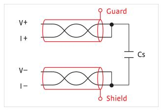
FIGURE 3-7 Capacitance Input shield and gard
