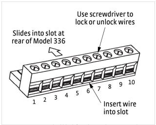
FIGURE 8-5 Terminal block for relays and Output 3 and 4
