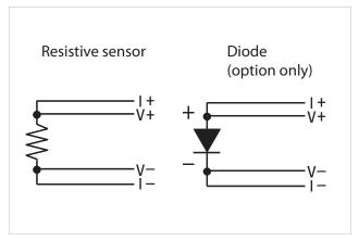
FIGURE 3-5 4-lead measurement
