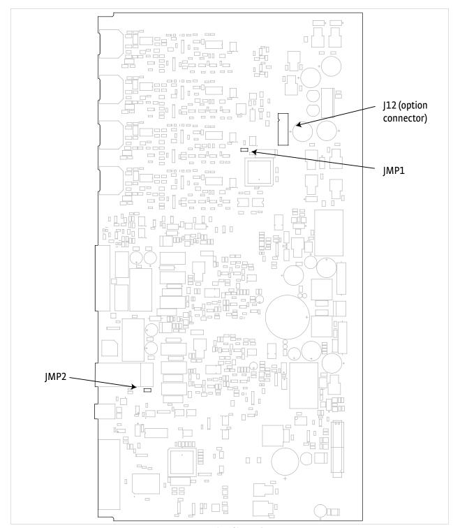
FIGURE 8-11 Location of internal components
