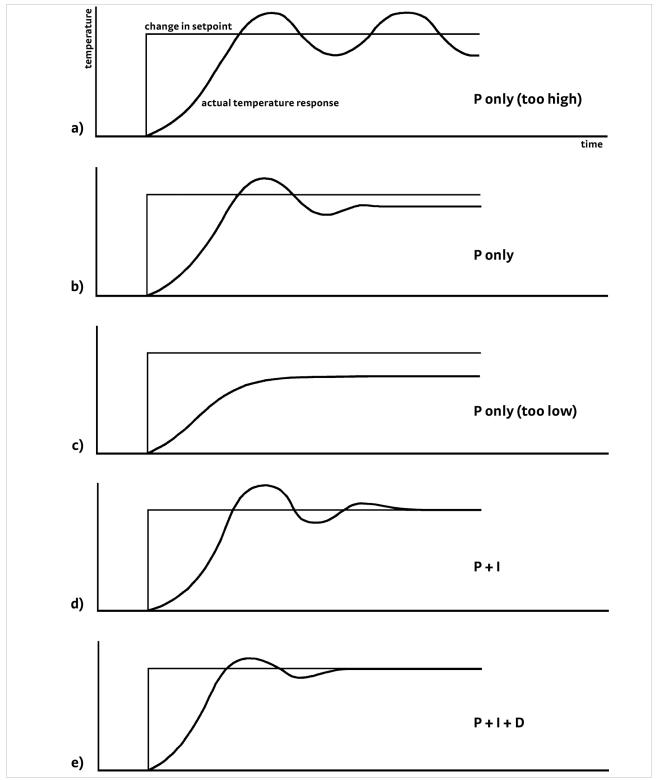
FIGURE 2-2 Examples of PID control
