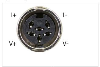
FIGURE 3-3 Sensor input connector
