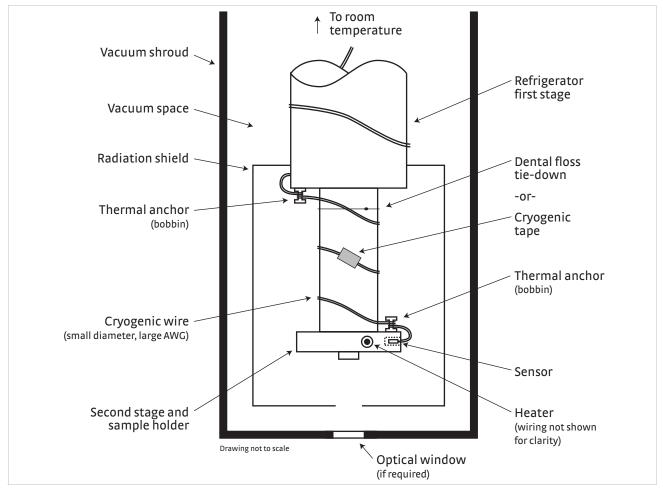
FIGURE 2-1 Typical sensor installation in a mechanical refrigerator
