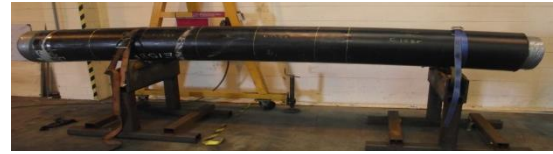
(a) Flexible pipe segment before FAT (pre-FAT)
