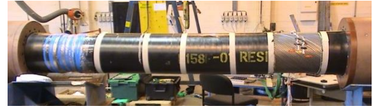
(b) Flexible pipe segment after FAT (post-FAT)
