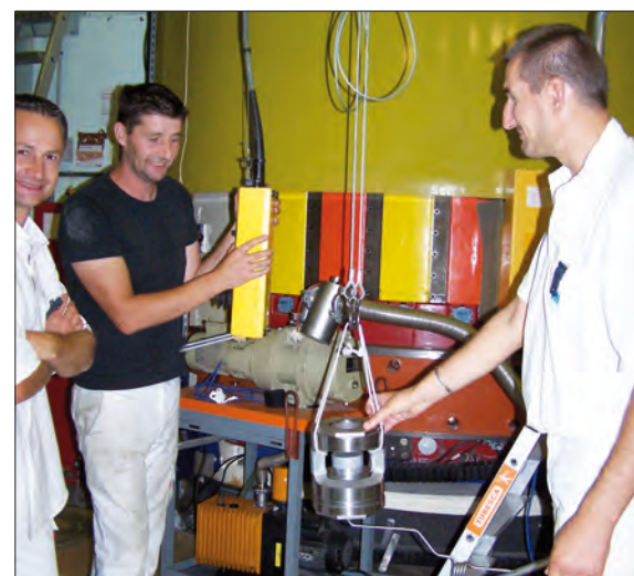
Figure 2: Removal of the Paris-Edinburgh press from the D4 bell jar at the end of a successful neutron diffraction experiment.
