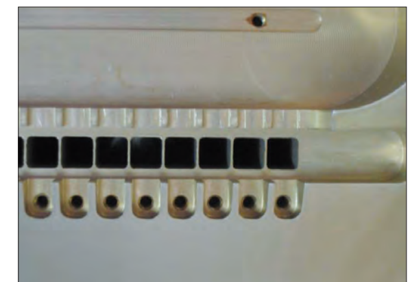
Figure 5: Detail of the new D17 MAM detector, showing the individual tubes tailored by spark erosion in a single block of aluminium.
