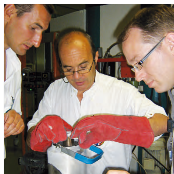
Ammonia monohydrate sample loading in the high-pressure cell directly at 77 K.
