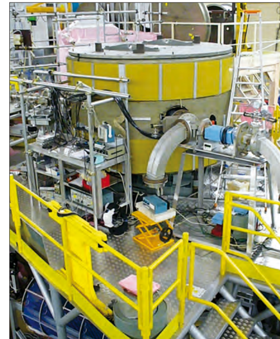
Figure 2: Double-chamber EDM spectrometer installed at ILL's UCN facility PF2.
