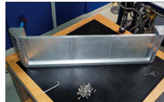
Figure 2: Small-size prototype of the D33 multitube MAM detector.
