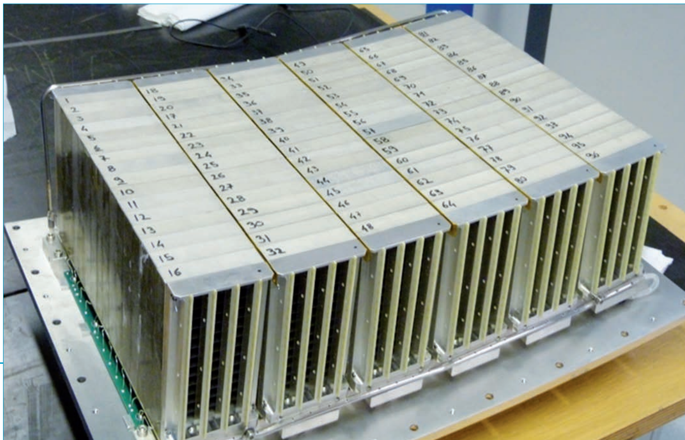
Figure 1: Inside view of the IN6 Multigrid prototype. Each of the 6 columns contains 16 grids and 60 proportional counters.
