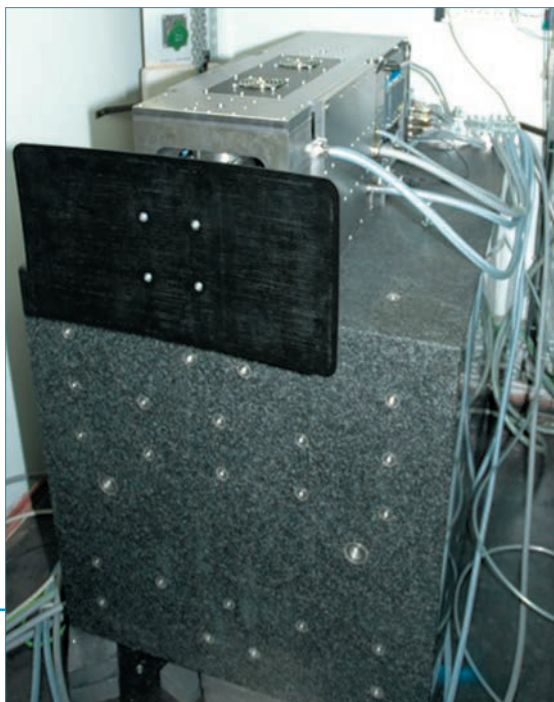
Linear motor Doppler drive for IN16B (built by AEROLAS) with the monochromator plate without crystals mounted.
