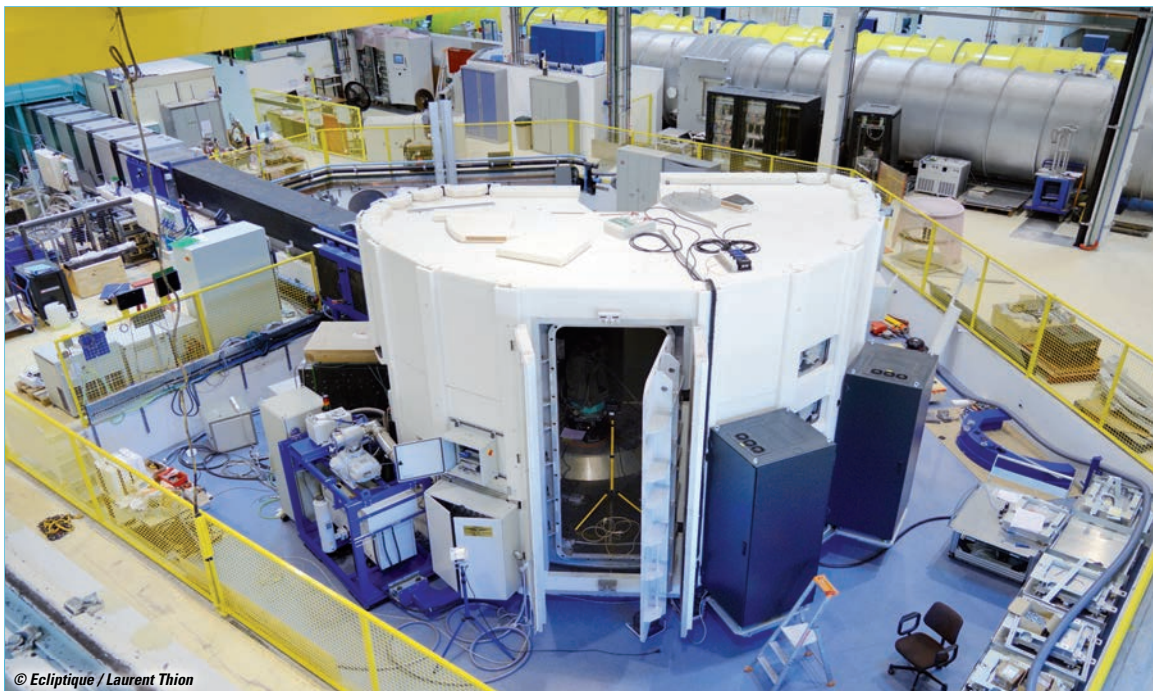
Figure 2: The new backscattering instrument IN16B.
