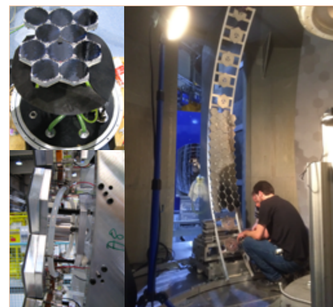
Figure 1 GaAs prototype. Top left: Monochromator, mounted on goniometers, with water cooling circuit and power supply. Bottom left: Side view of an analyser segment, with alignment mechanics and temperature control. Right: Analyser mounted inside the spectrometer. (Photos: Markus Appel, Bernhard Frick)
