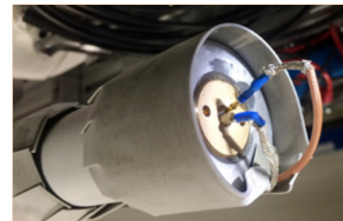
Figure 3 Picture of the assembled cell seen from the bottom. It shows the cadmium shielding and the connection point where coaxial cables plug the electronics into the dielectric capacitor.
