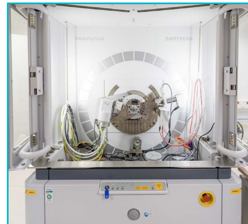
X-ray diffraction bench (IRT-Nanoelec).
